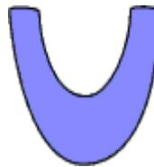
In those days (1966) gouges were all forged by hand and came in all shapes and sizes. They were all carbon steel as HSS gouges were not yet available. They had to be reground often and I used up quite a few. This is a typical section of a carbon steel forged gouge. I began to experiment with a view to making the gouge last longer between sharpenings and also
