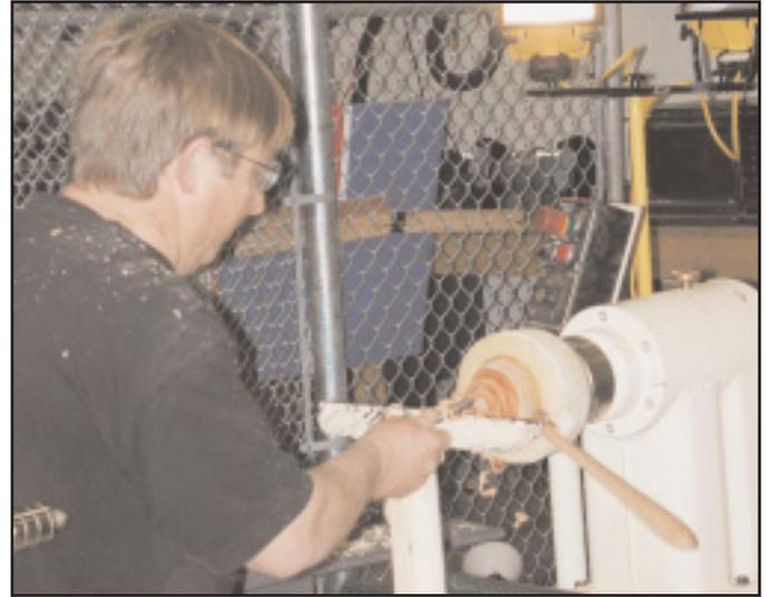
*Turning the bowl of a spoon in a jam chuck.*
