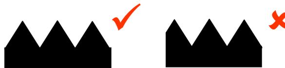
**Step 4:** Dull the leading edge of the chaser. When you ground off the partial threads you very likely “sharpened” the top of the chaser so now it is like a scraper. In the process of chasing you often bottom out again a surface that you do not want to cut, so just grind or file the end of the threads so they are dull.
