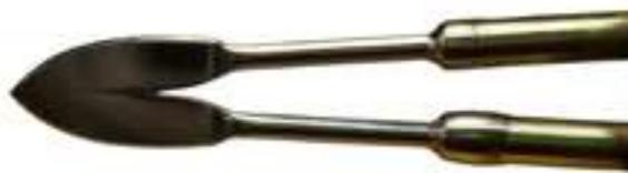
Here is an **example of a spear-point, round-heel burning tip.**
