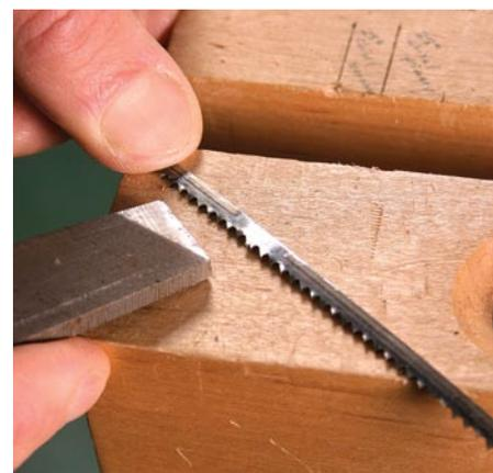
**6** The final step is to file off the burrs at the joint and remove the glass-like residue left by the flux.
