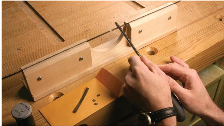
**2** Align the two ends of the sawblade in your jig. Sight across the blade and use a screwdriver to tap the ends into position.
