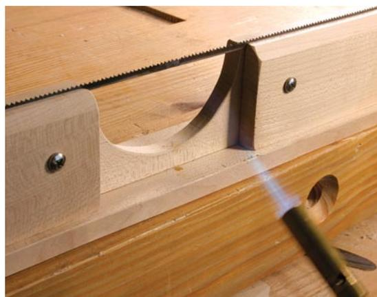
**5** Remove the brittleness from the band by heating the joint using successively less and less heat. Back up the torch on each pass.
