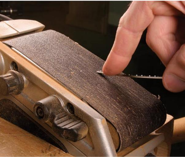
**1** Cut your band  $\frac{1}{4}$ " longer to allow for the overlap at the joint. Here we're using a belt sander to bevel one end of the band to create the scarf joint.
