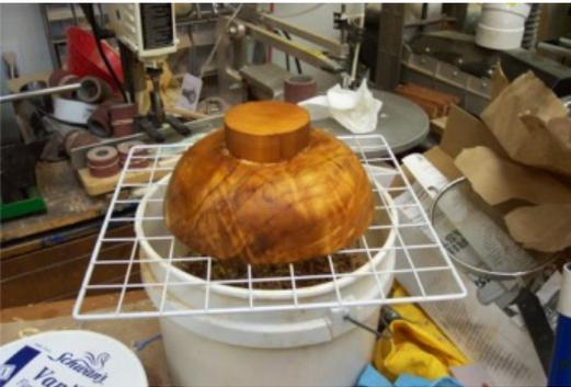
Remove the blank from the alcohol and let it air dry for about an hour to dry the surface.
