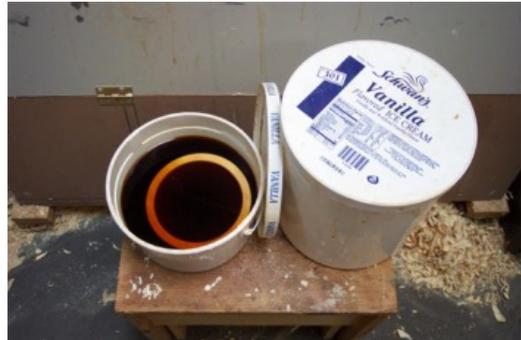
ensure good penetration of the alcohol. Longer soaking time does not appear to damage the wood.
