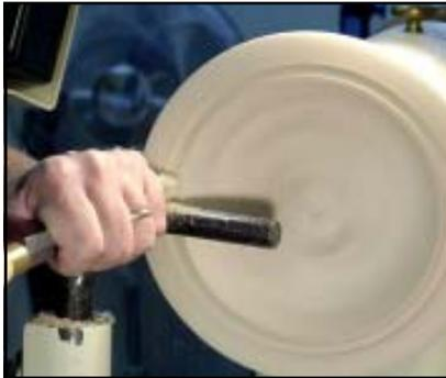
**Step 2** Remove the wood between skew lines with a cutoff tool to a depth of about 3/16".
