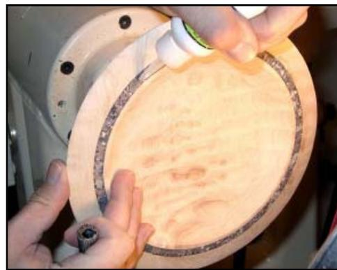
Progress through finer grits of sandpaper finishing the entire piece. If a large void occurs remove the wood plus chuck and repair, otherwise fill small voids with thick CA glue.
