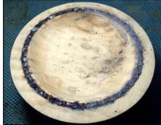
The stone glued-up with finer crushed material added around the coarser pieces. Tap the wood gently settle the material then add superthin CA glue.
