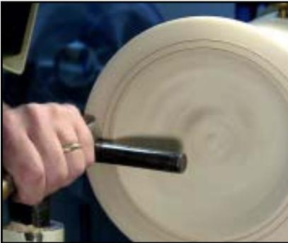
**Step 1:** Pretrim the inlay band notch with a skew chisel to a depth of about 1/4".
